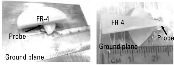
Figure 2.52 Stacked and segmented fabricated antenna structure [85].
