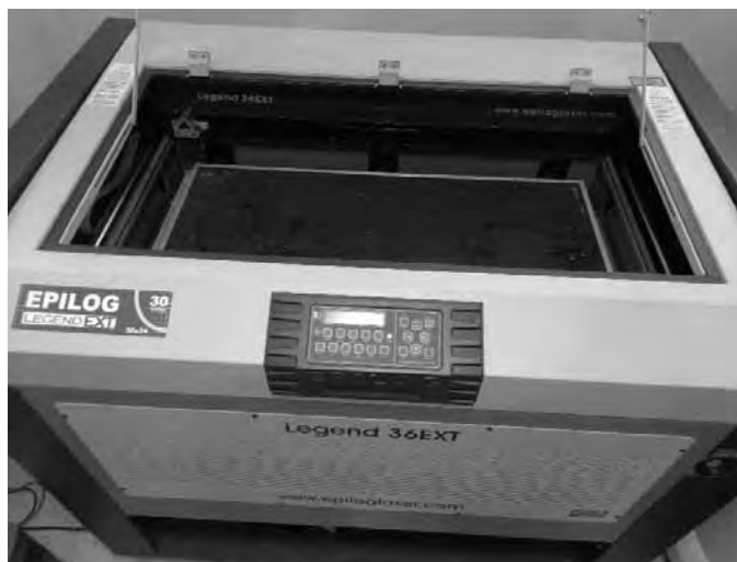
Figure 6.4 A laser cutting machine for cutting thin substrates.
