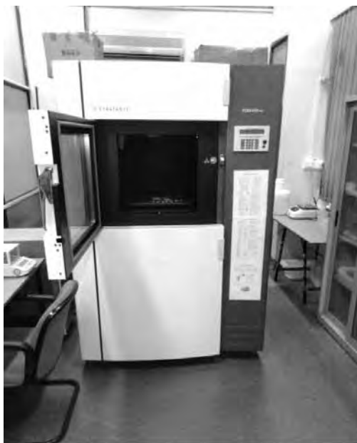
Figure 6.5 A 3-D printer as a tool for additive manufacturing available at the mechanical workshop of IIITDM Jabalpur.
