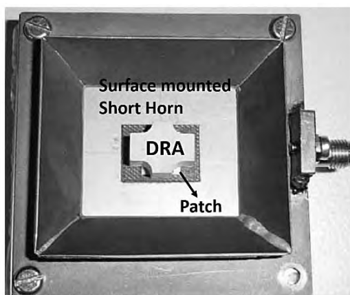
Figure 4.16 Proposed DRA configuration with a fabricated prototype of a short horn [24].
